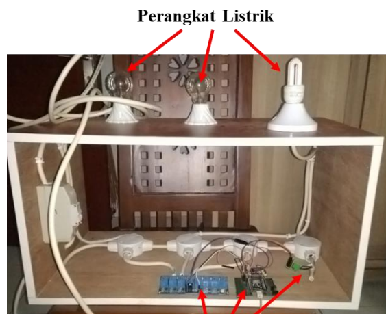
Modul Relay, NodeMcu, ACS712
